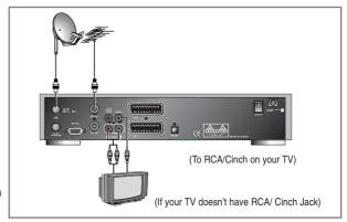
3. Finally connect the coaxial cable from the LNB to the LNB IN jack on back of the STB.
